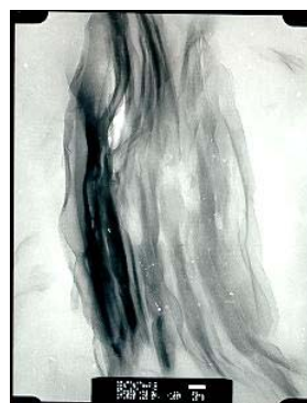
Figure 4. Transmission electron micrograph of the PVB/clay film. Scale bar 100nm.
