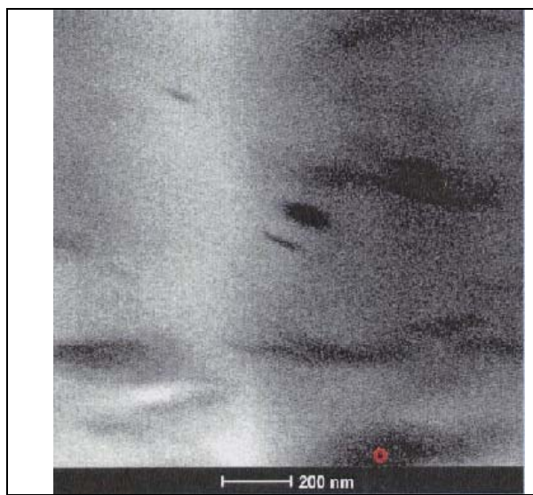
TEM image of a thin film sample of Nanomer C.30PE composite with 3% wt MMT at 60 rpm.
