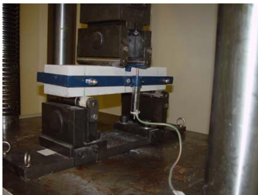
Figure 2. Flexural test set-up
