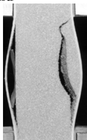
Figure 4. Compression failure of a sandwich specimen with implanted F/C debond.
